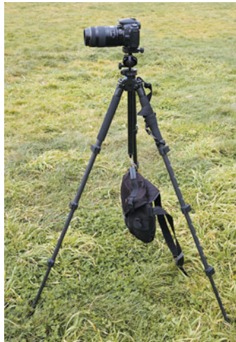
FIGURE 9.3 For extra stability in this shot, we've attached the weight hook to the bottom of the camera, and hung our camera bag from the hook. Note, too, that we have not elevated the center column.
